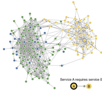
Fig. 1. SAP-managed service dependencies of a large organizational unit. Node color encodes native cloud environment of a service. Two large clusters correspond to the older (yellow) and newer (green, blue) environments.
